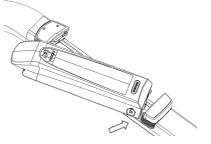
2. Push the battery into the battery holder, when hears a 'click' sound, that means battery is locked.
